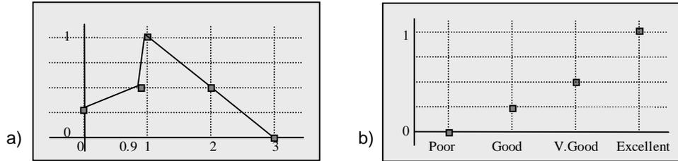
Figure 5. Satisfaction functions: a) for the Price attribute  $S(1)=1$ ,  $S(2)=S(0.9)=0.5$ ,  $S(0)=0.275$ ,  $S(3)=0$  and b) for a Quality attribute, for which values are an ordered set of labels.
