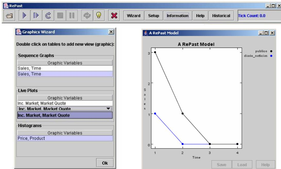
Figure 6. Top: Simulation toolbar (RePast enhanced) includes buttons such as Start, Step, Stop, Wizard for output definition (opened in bottom left side), Agent Information, Historical Information, or Tick Display. Bottom right: sequence graph showing a simulation output of sales along time.
